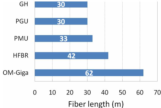
Fig. 5. Length limits for the tested fibers when transmitting GbE data (1.25 Gb/s, PRBS  $2^7-1$ ).
