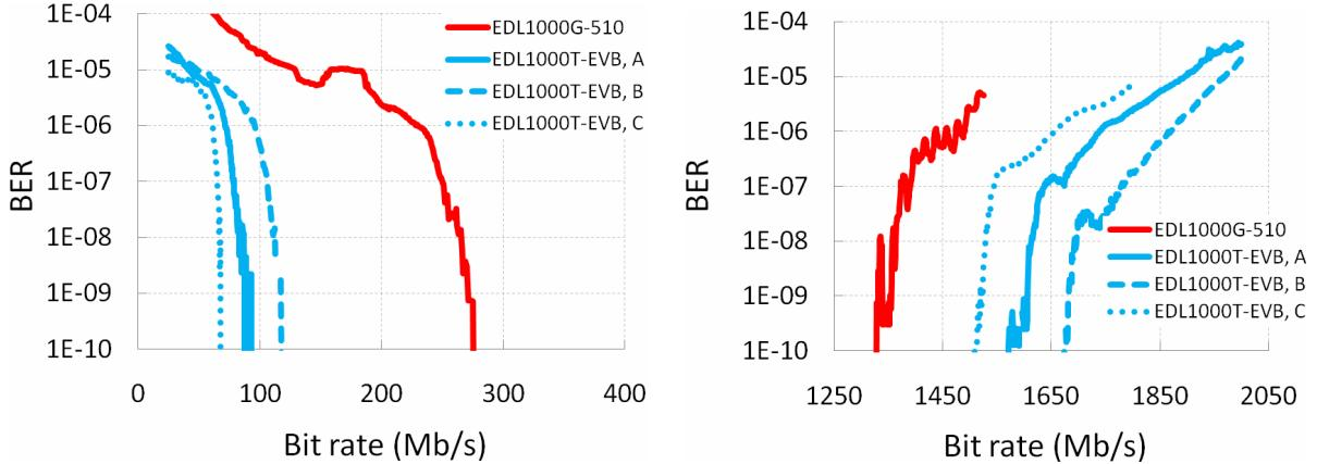
Fig. 2. Error-free limits for lower data rates (left) and upper data rates (right) for the prototype EDL1000G-510 (red) and three different samples of EDL1000T-EVB (blue) using a PRBS  $2^{23}-1$  data pattern.
