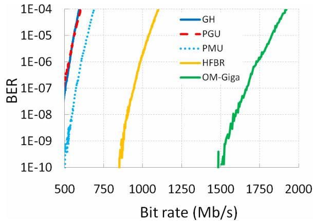
Fig. 4. Bit rate limits for 50 m of the tested fibers, PRBS 2<sup>7</sup>-1 data pattern.
