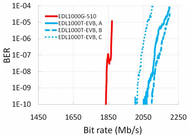
Fig. 3. Error-free limits for upper data rates for the prototype EDL1000G-510 (red) and three different samples of EDL1000T-EVB (blue) using a PRBS  $2^7-1$  data pattern.
